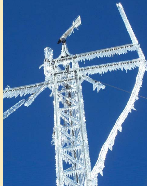
A brilliant combination of sunlight and ice bathes the Kingfisher Mesonet station on February 1st, 2002. The ice observed on the guy wires (hanging below and to the left of the station) approached the diameter of a soft drink can. Photo by Chris Fiebrich.
