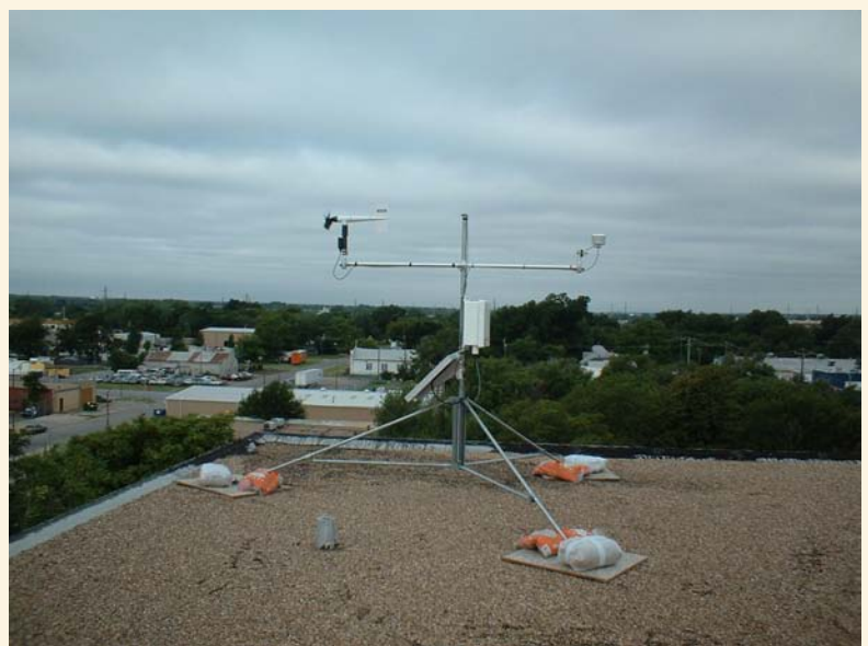
Figure 2. A rooftop mounted weather station mounted during Joint Urban 2003.
