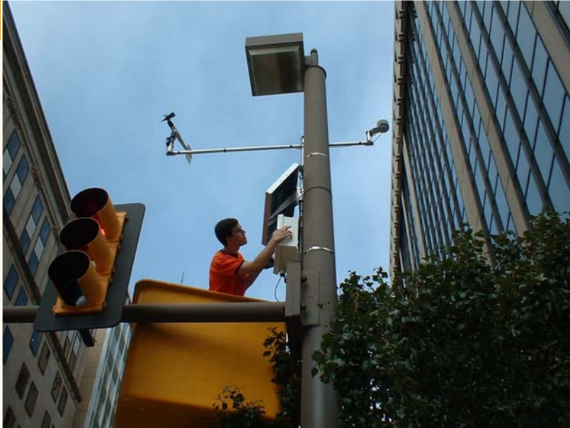
Figure 1. A weather station mounted on a traffic pole during Joint Urban 2003 (Peter Hall from OCS is pictured).
